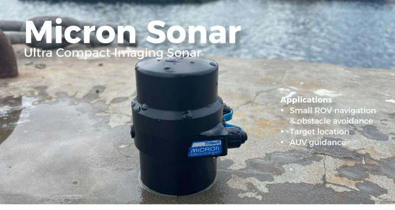
The Tritech Micron Sonar has set high standards in compact sonar technology. It is one of the smallest digital CHIRP sonar in the world. CHIRP technology dramatically improves the range resolution compared with conventional sonars and is a feature normally associated with much larger, more expensive systems.
