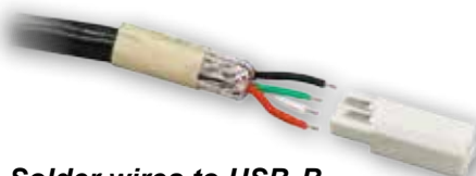
Solder wires to USB-B Insert
