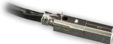
Install insert, attach lid, and crimp shield
