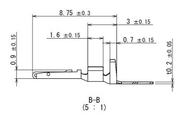
NOTE1. CONTACTS ARE SUPPLIED IN REELED FORM WITH 9000 CONTACTS PER REEL. NOTE2. APPLICABLEWIRE DIMETER : AWG#24 $\sim$ #28、INSULATION DIA :  $\phi$ 0. 9 $\sim$   $\phi$ 1. 6 NOTE3. MARK TRADE NAME AND NO. OF CONTACTS.
